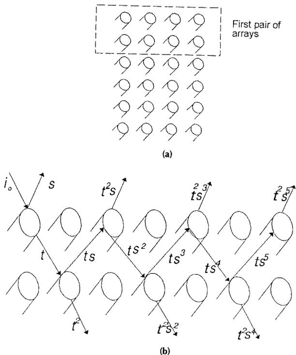
**Figure 1** (a) Cross section through a model of dyed cylindrical fiber. (b) Representation of grouping of the first pair of absorbing-scattering arrays.
