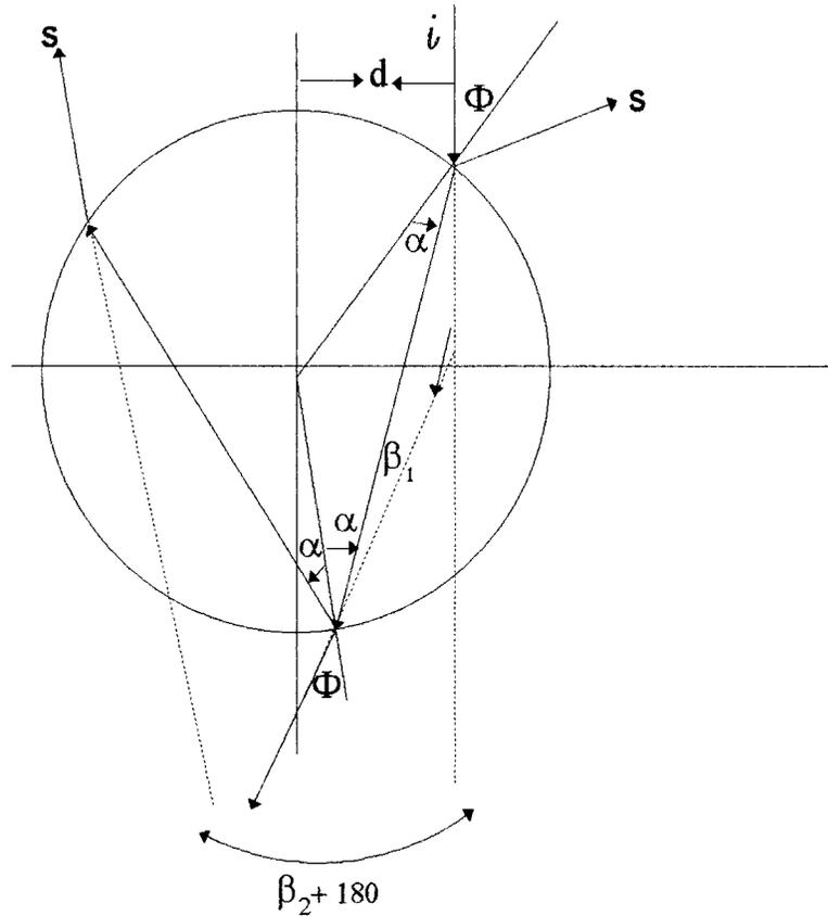
**Figure 2** Cross section through a fiber showing the different light reflections and refractions.
