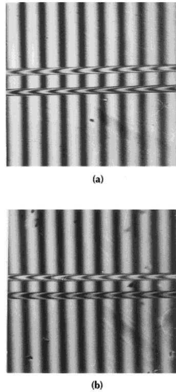
**Figure 3** Totally duplicated images using the Pluta interference microscope with monochromatic light of wavelength 546 nm, of fibers dyed with (a) Terasil red and Disperse yellow and (b) Novester blue and Terasil red.
