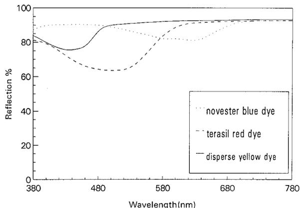
**Figure 5** Reflectance of polyester fibers dyed with Terasil red, Disperse yellow, and Novester blue dyes.
